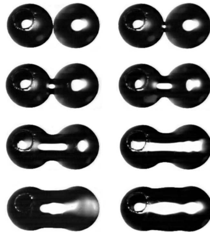
FIG. 2. Coalescence of a droplet pair (distilled water, initial radii R_0 = 2.5 mm) as viewed from directly above, at times 0, 0.777, 1.888, 4.111, 6.33, 8.55, 16.33, and 60 ms.
